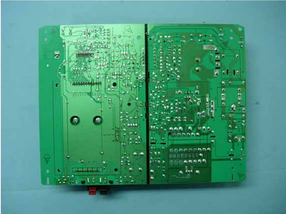
Figure 8 Internal View (Main Board, Back View)
