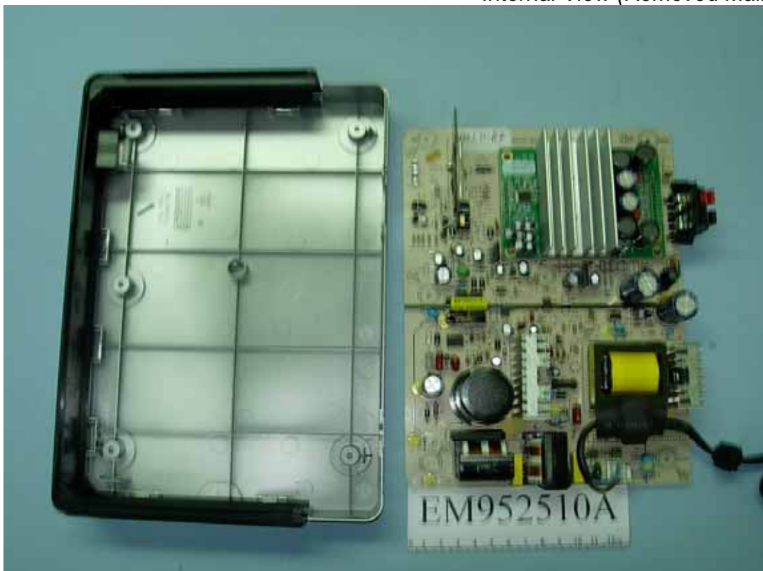
Figure 5 Internal View (Removed Main Board)
