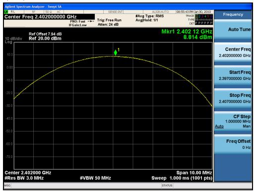
Test Plots (π/4DQPSK) Peak Power (CH.39)
