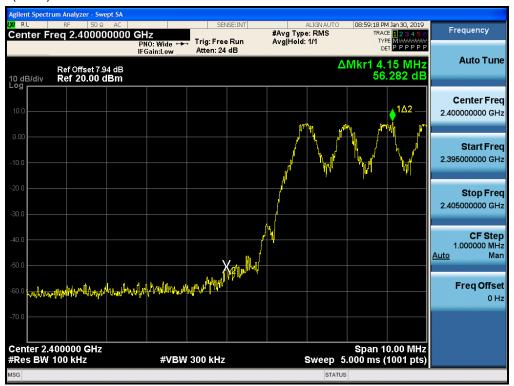
Test Plots with hopping (GFSK) Band Edges (CH.78)
