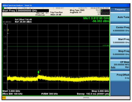
Test Plots (8DPSK)- 5 GHz - 7 GHz Spurious Emission (CH.0)
