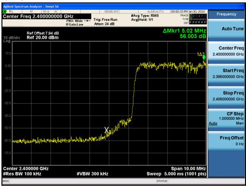
Test Plots with hopping (π/4DQPSK) Band Edges (CH.78)
