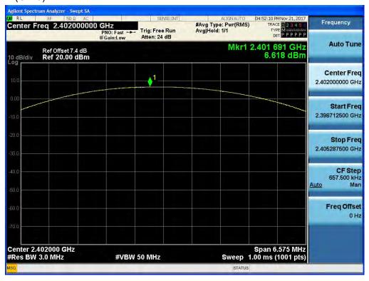
Test Plots (π/4DQPSK) Peak Power (CH.39)
