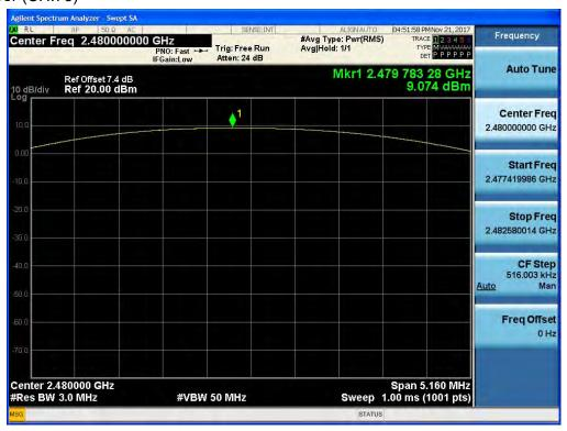
Test Plots (8DPSK) Peak Power (CH.0)
