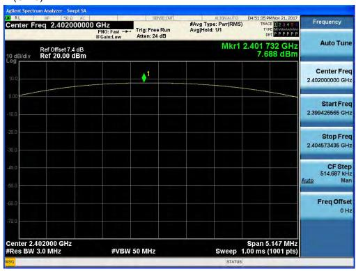
Test Plots (GFSK) Peak Power (CH.39)
