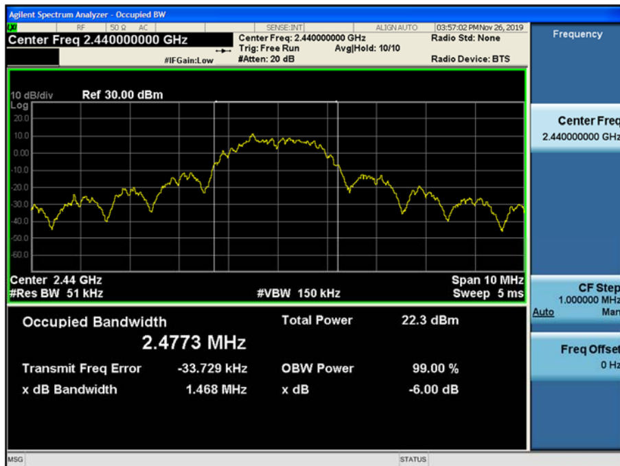
99% Bandwidth plot (CH 18)
