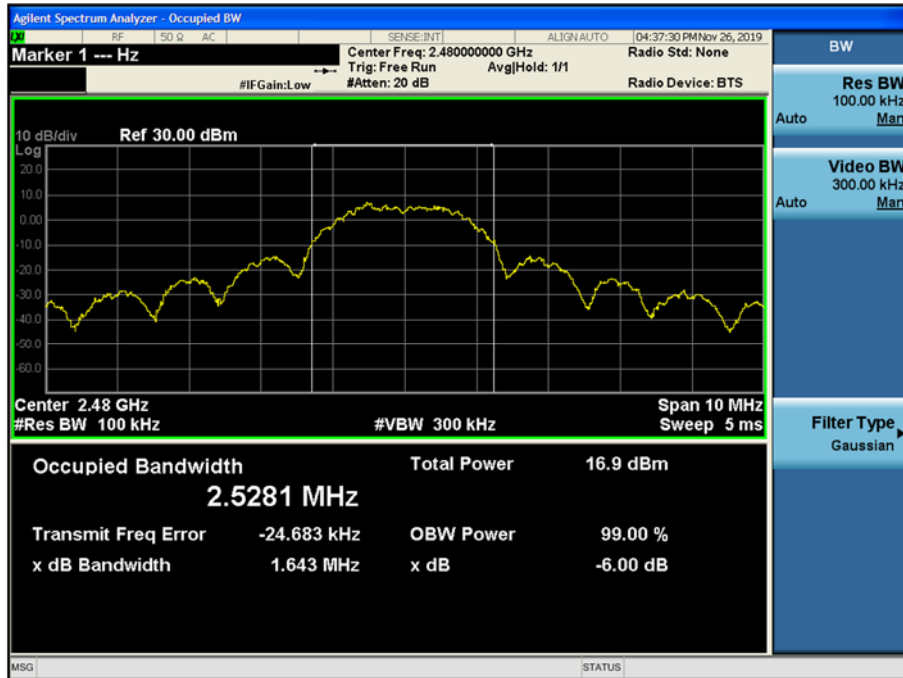
6dB Bandwidth plot (CH 26)
