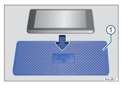
Fig. 131 Illustration: stowage area with mat for wireless charging function.
