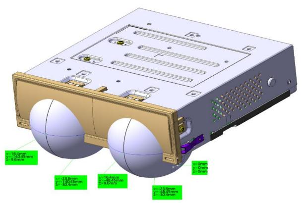
2 Sphere area are virtual space for showing a distance of 4cm from the radiator (from BT/Wifi ANT on PCB)
