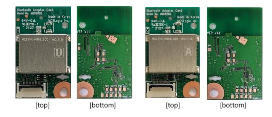
This MB8811QD Module is compatible with Bluetooth specification version 4.2. MB8811QD is a fully integrated RF, baseband controller etc.
