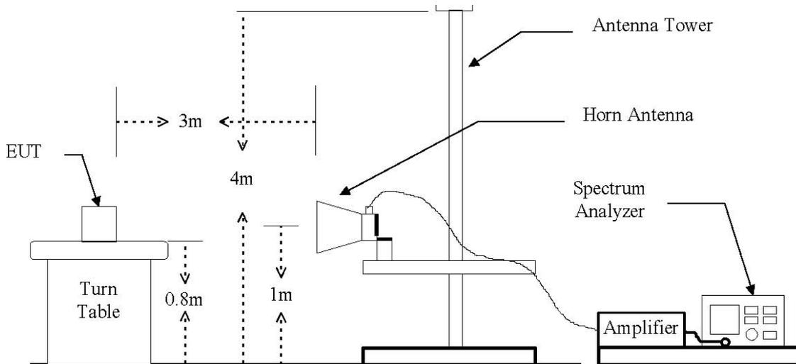
The diagram below shows the test setup for substituted method.
