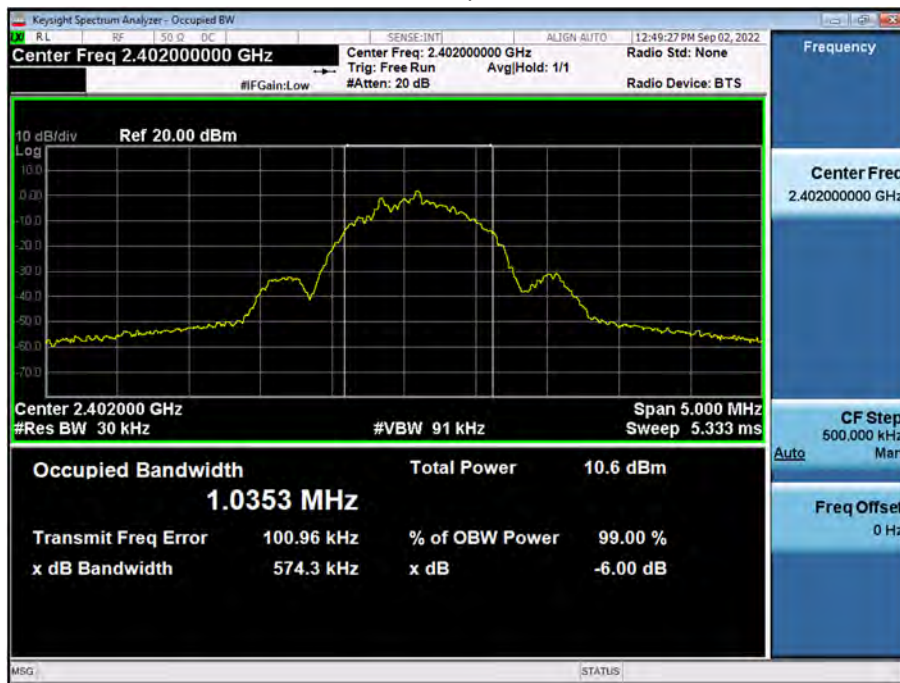
99 % Bandwidth plot (Low-CH 0)
