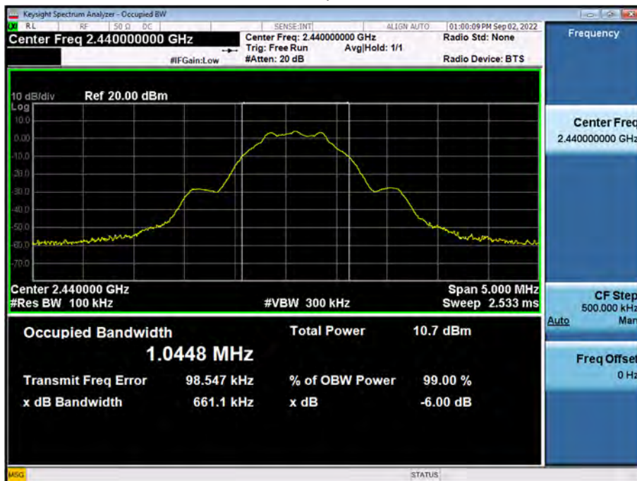
6 dB Bandwidth plot (Mid-CH 19)
