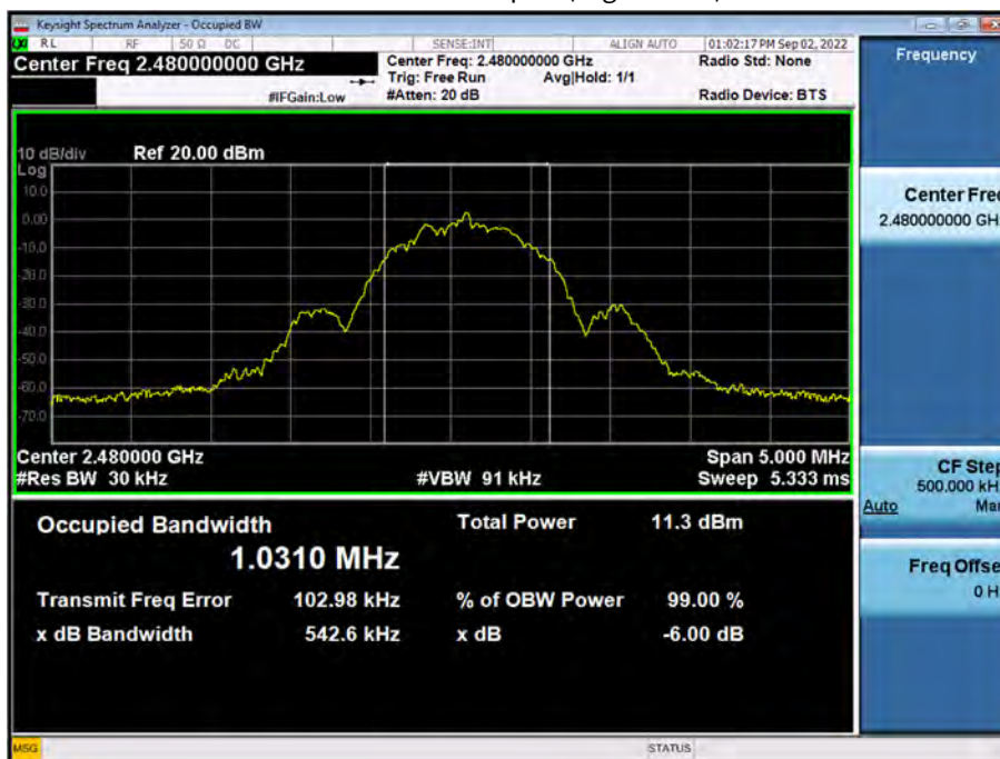
99 % Bandwidth plot (High-CH 39)
