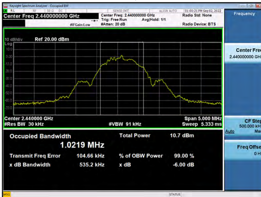
99 % Bandwidth plot (Mid-CH 19)
