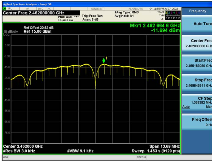
Power Spectral Density (802.11b - Ch. 11)
