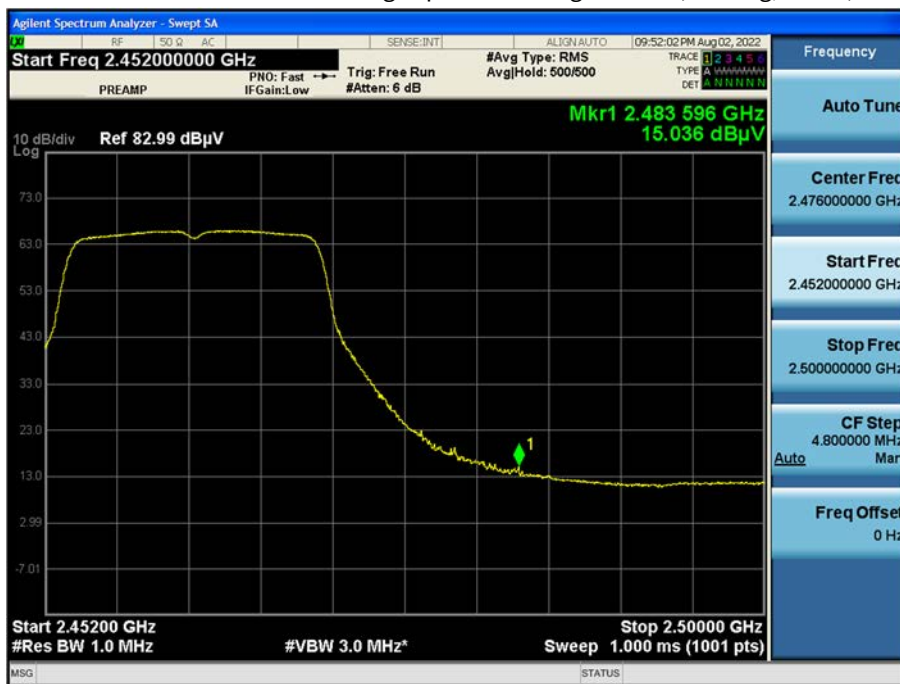
Radiated Restricted Band Edges plot – Average Result (802.11g, Ch.11)
