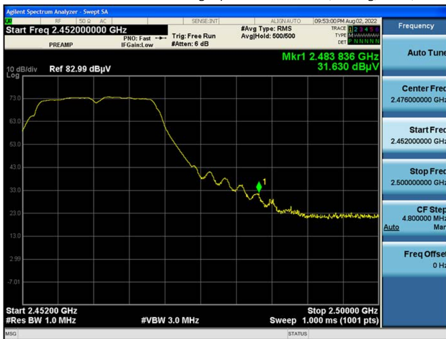
Radiated Restricted Band Edges plot – Peak Result (802.11g, Ch.11)
