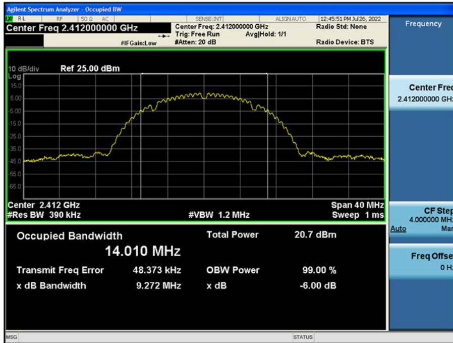
99% Bandwidth plot (802.11b-CH 1)
