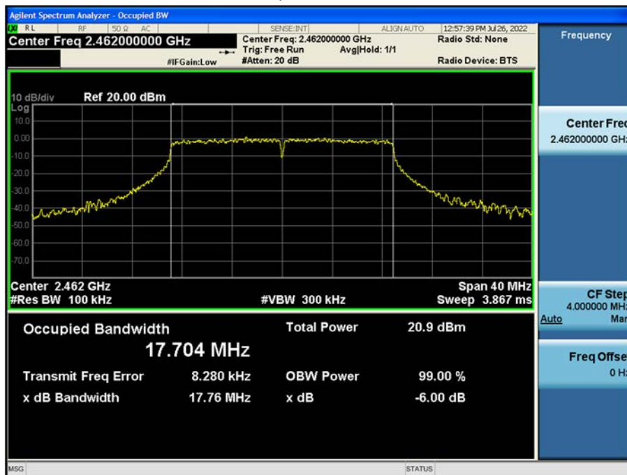
6dB Bandwidth plot (802.11n_HT20-CH 11)
