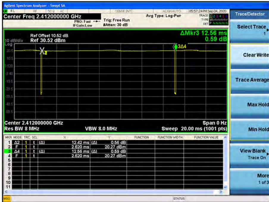
Duty cycle plot (802.11b(1Mbps))
