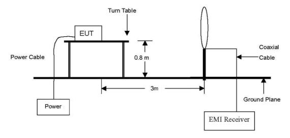
The diagram below shows the test setup that is utilized to make the measurements for emission from 30  $\,\rm Mz$  to 1  $\,\rm Gz$
