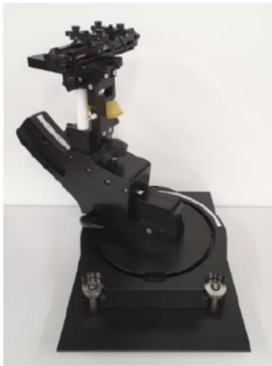
Figure 5.5 Mounting Device for Hand-held Devices and Laptop / Body-Worn Devices
