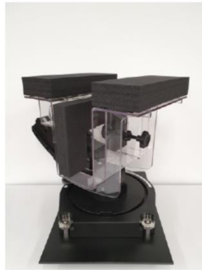
Figure 5.5 Mounting Device for Hand-held Devices and Laptop / Body-Worn Devices
