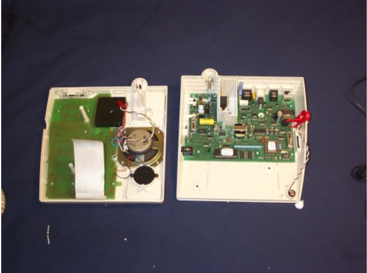
Photo 3: Top cover removed from EUT showing circuit boards. (Board on left is keypad circuit board. Board on the right is the main board)
