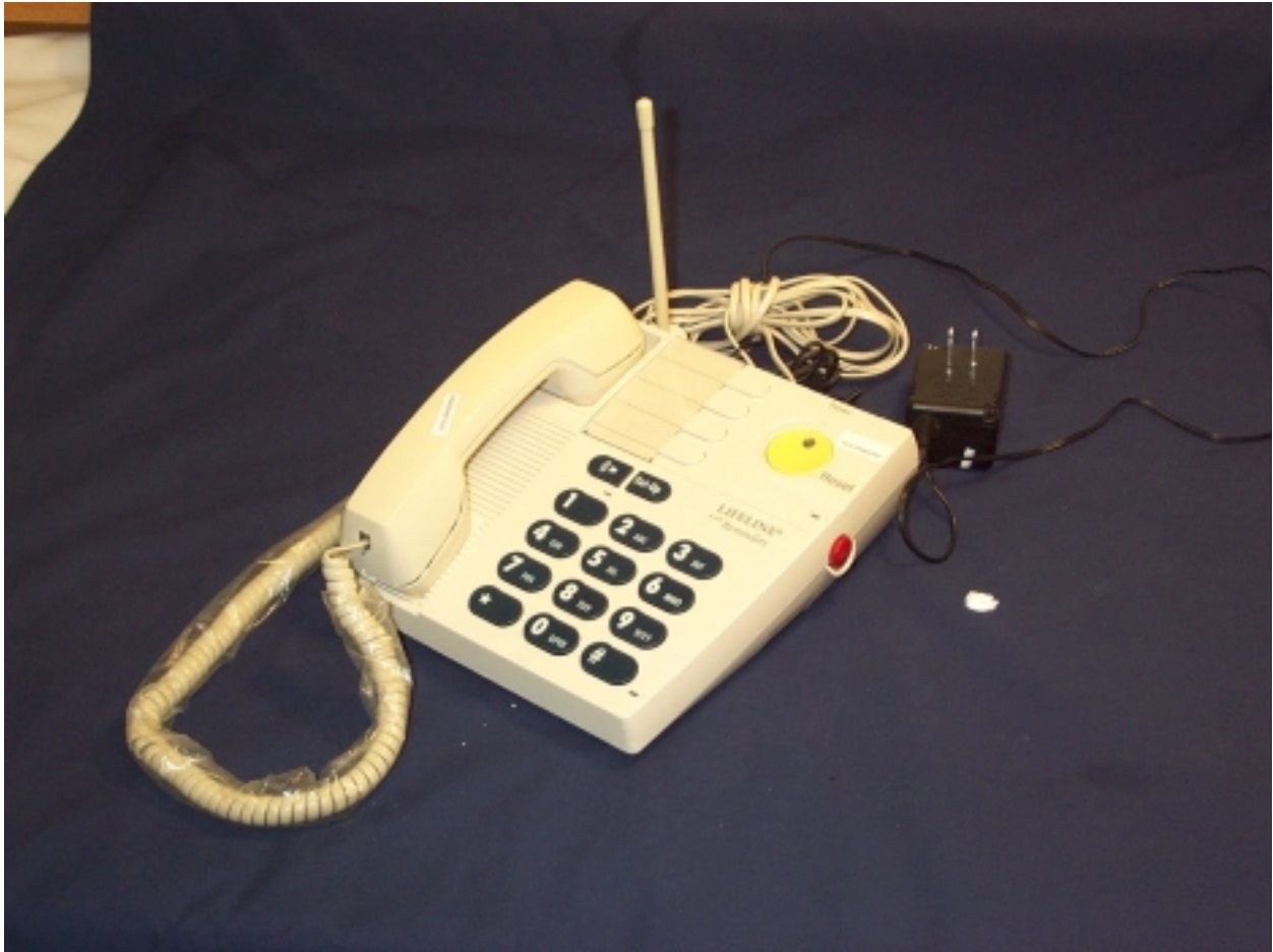
Photo 2: Oblique of 9500, showing RJ-11 POTS connection cable and “cube” style wall x-frmer.
