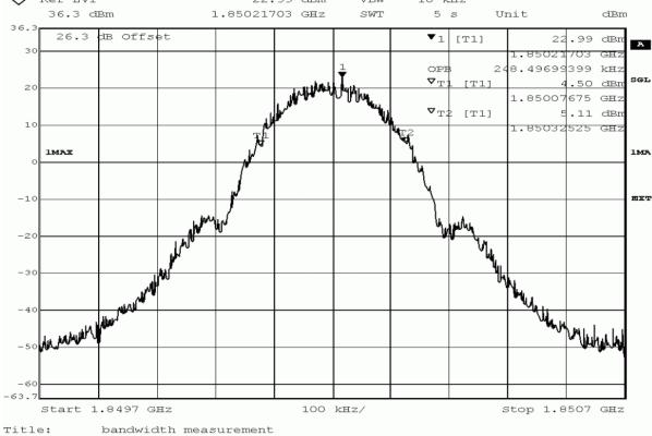
DE1015001, GSM1900, occupied bandwidth (99%), channel 512 (1850.2MHz)
