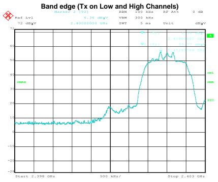
The emission at band edge is found to be 20dB lower than the fundamental
