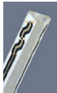
Figure 2.3 Probe Thick-Film Technique
