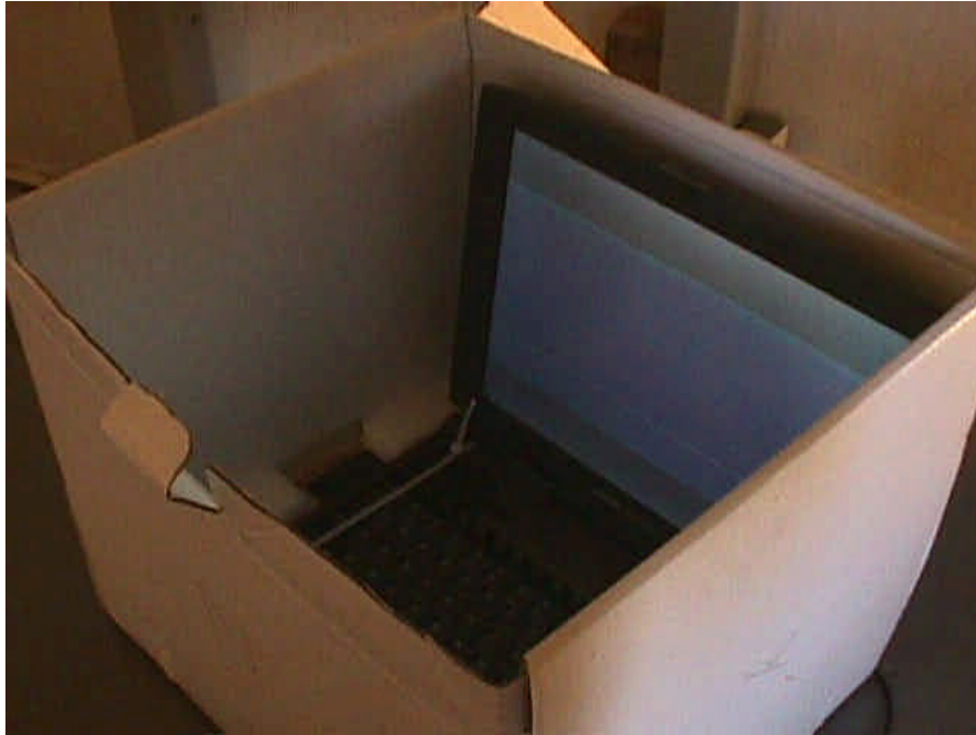
Radiated Emissions Test Setup (other antennas)
