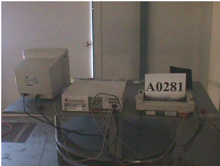
Radiated Emissions Test Setup (13 dBi antenna)
