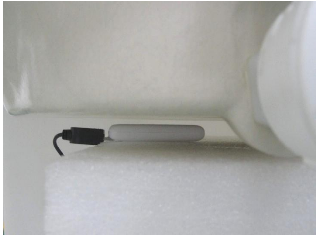
USB Cable Plug-in for USB Configuration 2 (Horizontal Down with Phantom 0.5 cm Gap)
