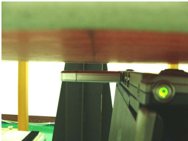
USB Configuration 1 for Back Off SAR (Horizontal Up with Phantom 1.0 cm Gap)
