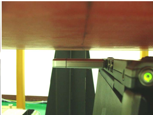
USB Configuration 1 for Back Off SAR (Horizontal Up with Phantom 1.5 cm Gap)
