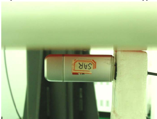
USB Configuration 4 with Cable (Vertical Back with Phantom 0.5 cm Gap)
