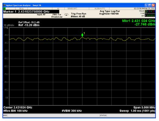
→ Power Spectral Density (Peak mode): -27.75 dBm
