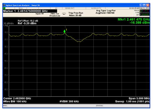
→ Power Spectral Density (Peak mode): -16.39 dBm
