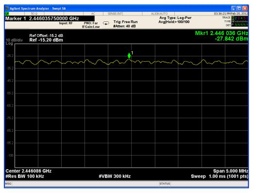
→ Power Spectral Density (Peak mode): -27.84 dBm
