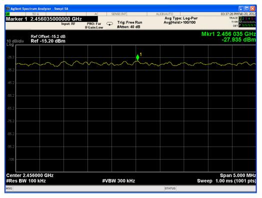
→ Power Spectral Density (Peak mode): -27.94 dBm
