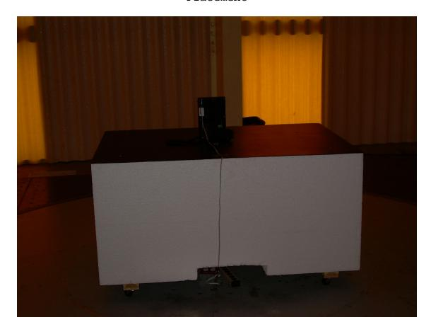
Front View Radiated Spurious Emissions Configuration - Vertical Placement
