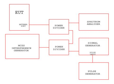
Test Configuration Block Diagram
