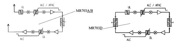
Downlink signals reach the duplexer. The duplexer is the frequency separation unit that splits and recombines uplink (UL) and downlink (DL).
