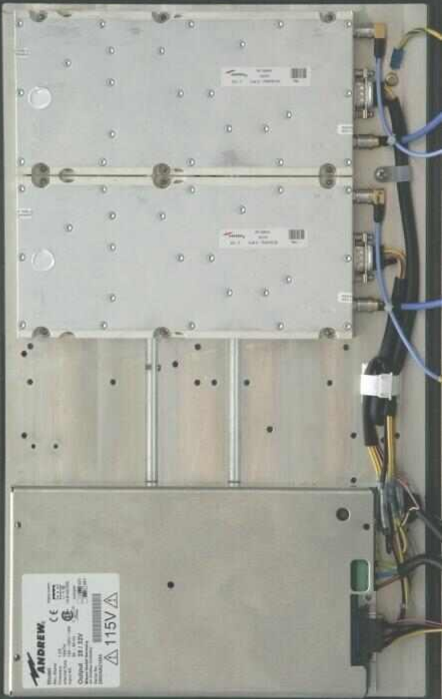
Main Unit - Power supply and PA assem.
