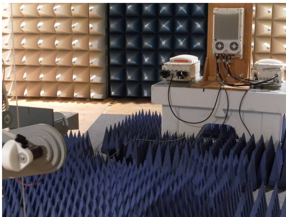
picture 8.4: Test setup: Field Strength Emission >20 GHz @3m in the FAC
