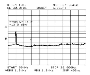
**Test Data – Spurious Emissions at Antenna Terminals** GSM
