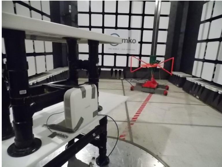
Figure 9.1-1: Radiated setup photo
