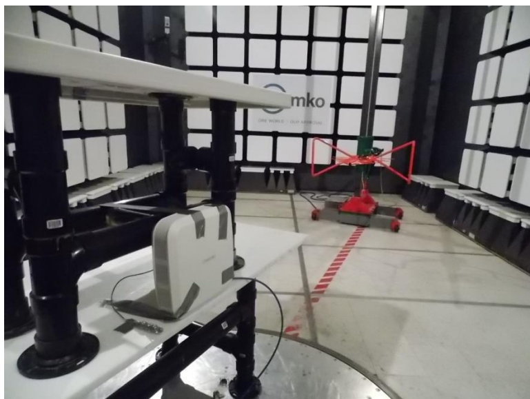
Figure 9.1-1: Radiated setup photo
