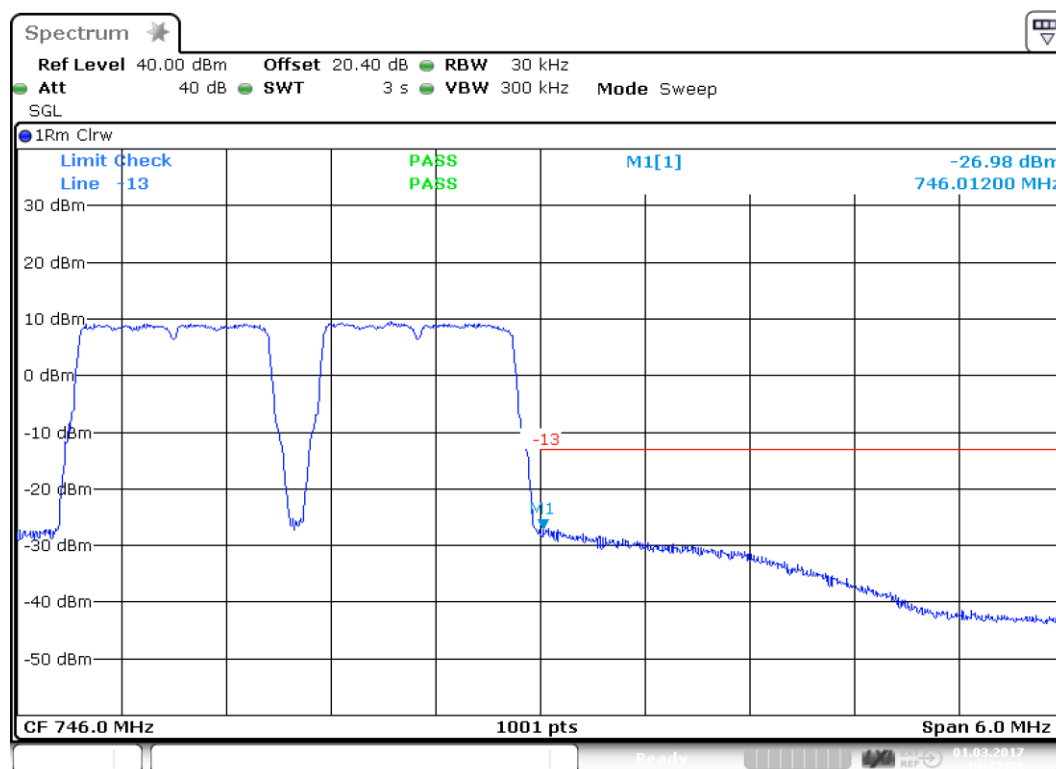
plot 8.3.2.1-#1 Intermodulation: §27.53, §2.1051; Test results; Downlink LTE 728 – 746MHz Lower Band Edge
