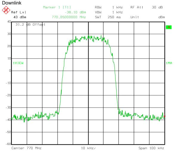
Occupied Bandwidth Input TDMA Downlink
