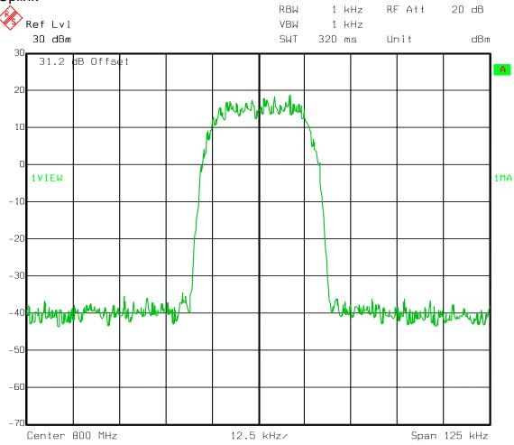
Occupied Bandwidth Input TDMA Uplink
