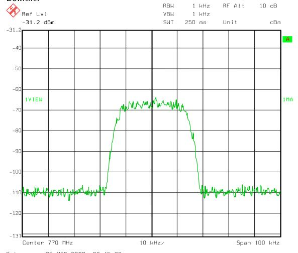
Occupied Bandwidth Output TDMA Uplink
