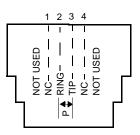
Table 2-6RJ-11 pinout specification
