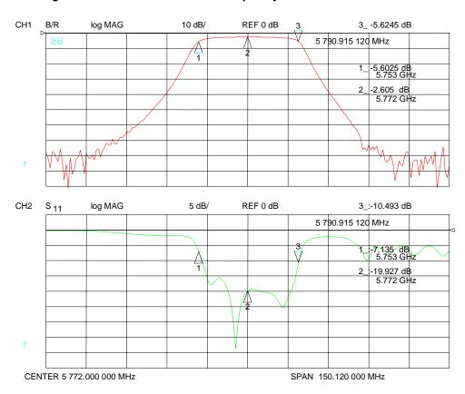
Figure A-8 Filter with center frequency of 5.772 GHz
