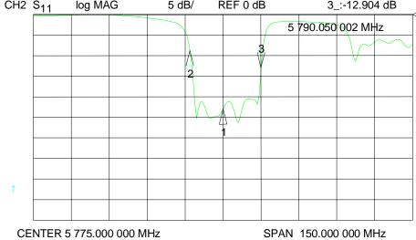
Figure A-3 Filter with center frequency of 5.775 GHz
