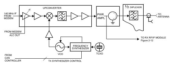
Figure 2-11 Upconverter and Power Amplifier block diagram
