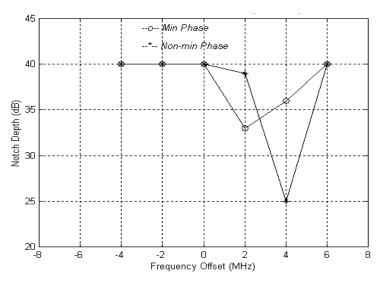
Figure E-5 W Curve at BER = 1E-6, Direction B
