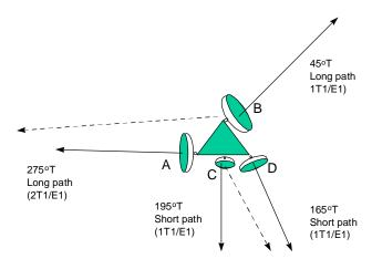
Figure 3-6 Tower mounting with no blockage
