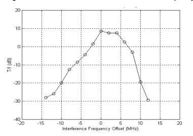
Figure C-7 T/I versus narrowband interference frequency offset
