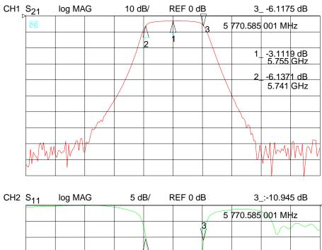
Figure A-2 Filter with center frequency of 5.755 GHz
