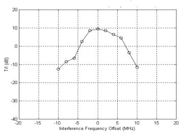
Figure C-10 T/l versus wideband interference frequency offset (Direction A: 05B8, Direction B: 0247)
