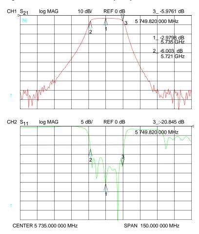
Figure A-1 Filter with center frequency of 5.735 GHz
