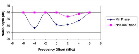
Figure D-5 W Curve at BER=1E-6, Direction B
