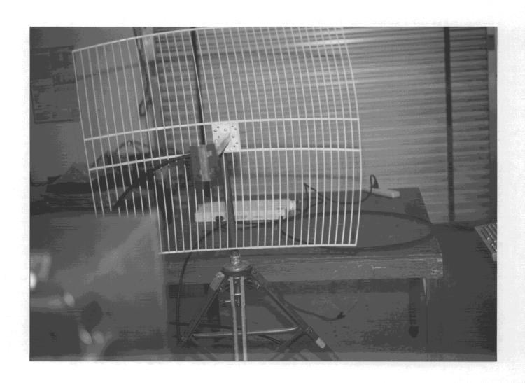
Figure 3. Another view. Photograph of Aurora 2400 Transmitting antenna and EMCE Receiving antenna setup for Radiated Emissions measurement. Test distance equals 1 meter. Aurora Radio on wooden table.
