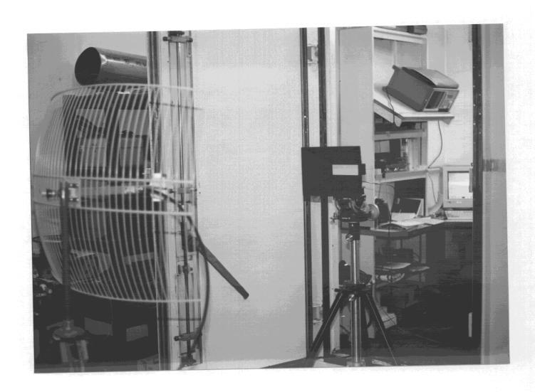
Figure 2. Another view. Photograph of Aurora 2400 Transmitting antenna and EMCE Receiving antenna setup for Radiated Emissions measurement. Test distance equals 1 meter.
