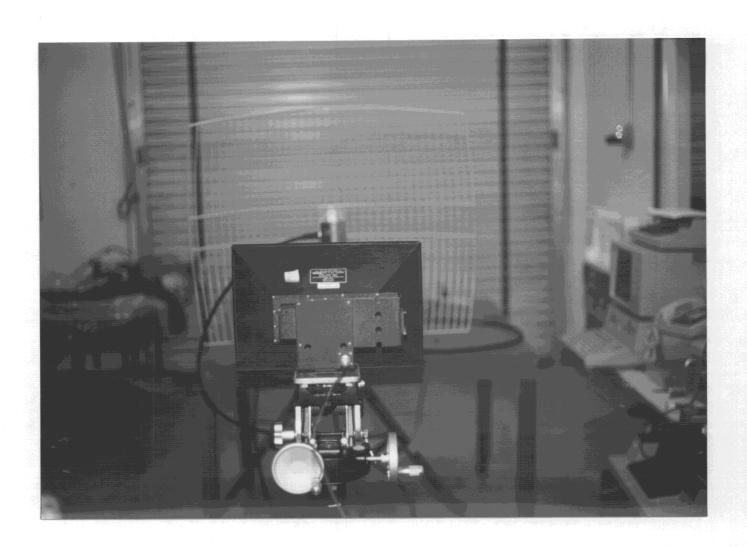
Figure 1. Photograph of Aurora 2400 Transmitting antenna and EMCE Receiving antenna setup for Radiated Emissions measurement. Test distance equals 1 meter.
