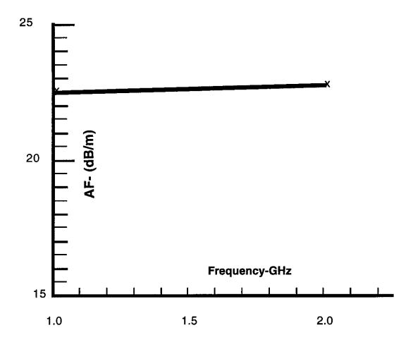
Figure 1. Antenna Factor for Polarad CA-L.
