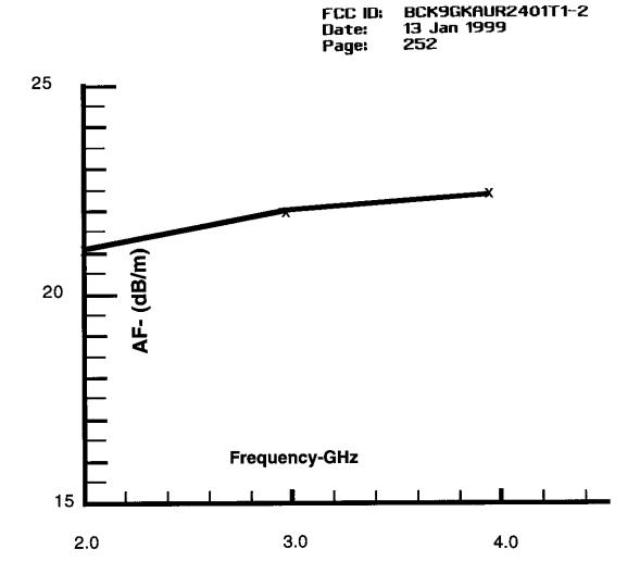
Figure 2. Antenna Factor for Polarad CA-S
