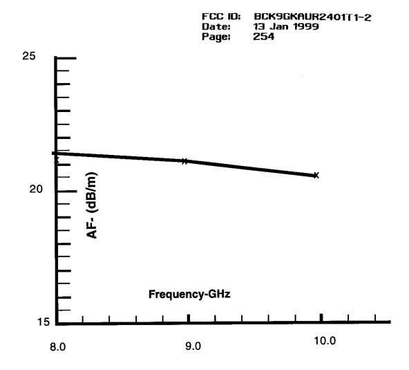
Figure 4. Antenna Factor for Polarad CA-X W/CA-R2 Reflector.
