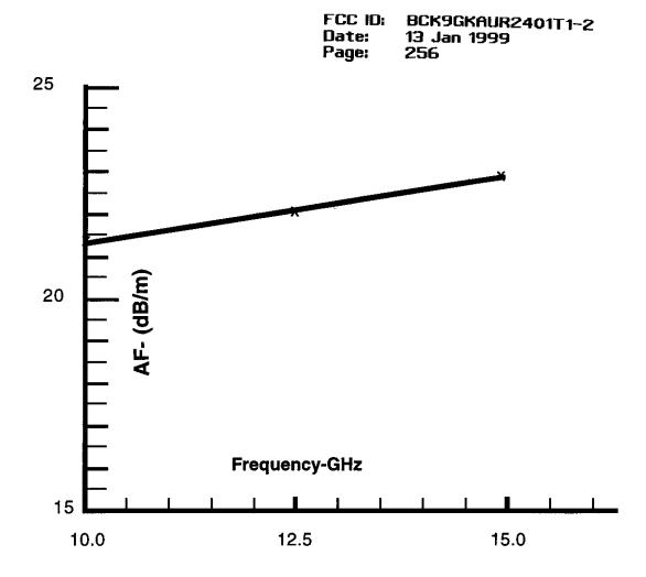
Figure 5. Antenna Factor for Polarad CA-KS W/CA-R2 Reflector.
