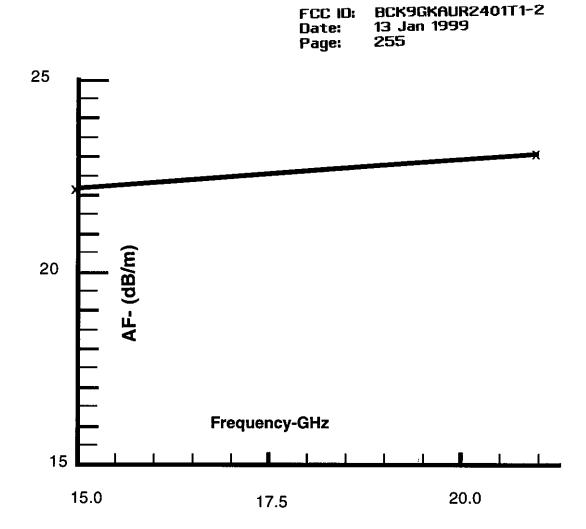
Figure 6. Antenna Factor for Polarad CA-KU W/CA-R2 Reflector.
