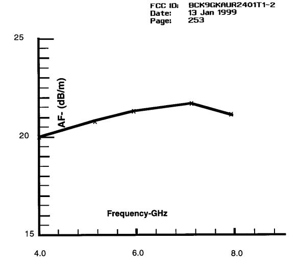
Figure 3. Antenna Factor for Polarad CA-M W/CA-R2 Reflector.
