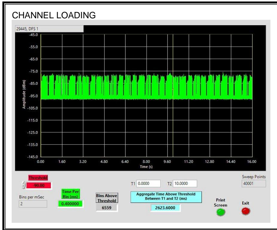
The level of traffic loading on the channel by the EUT is 26.23%
