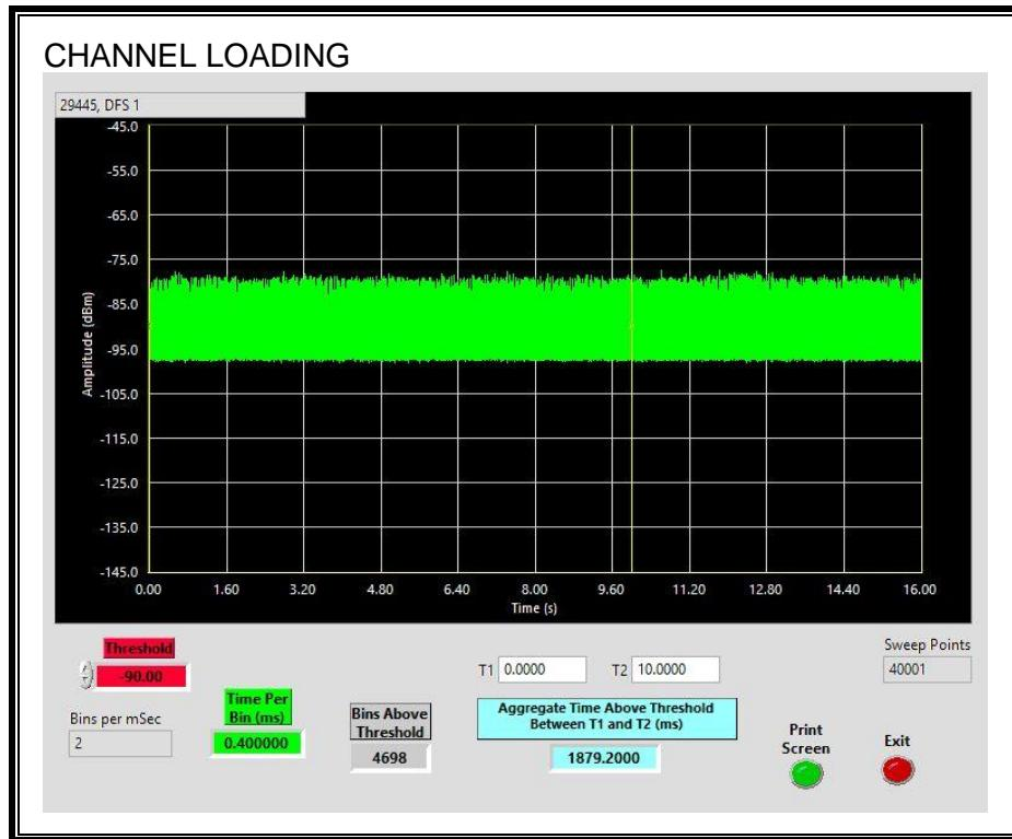
The level of traffic loading on the channel by the EUT is 18.79%
