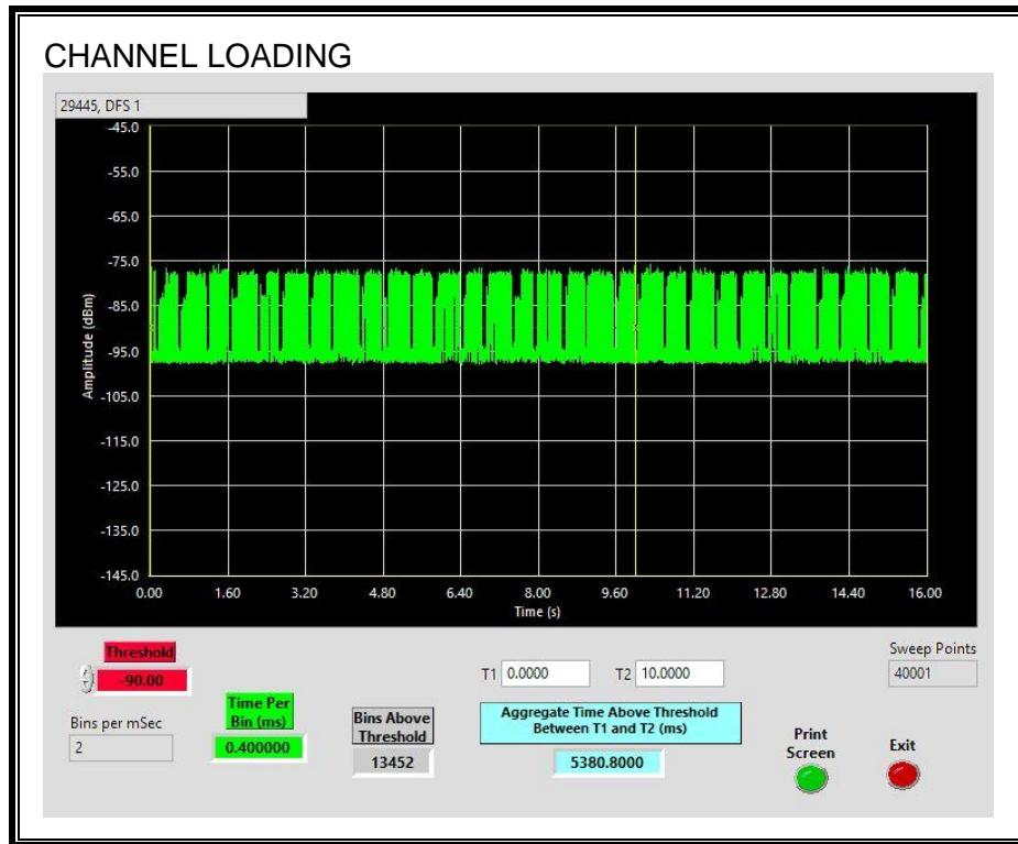
The level of traffic loading on the channel by the EUT is 53.8%
