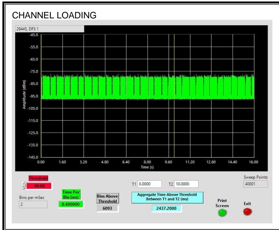
The level of traffic loading on the channel by the Peer Slave is 24.37%.
