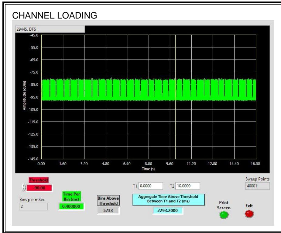
The level of traffic loading on the channel by the Peer Slave is 22.93%.
