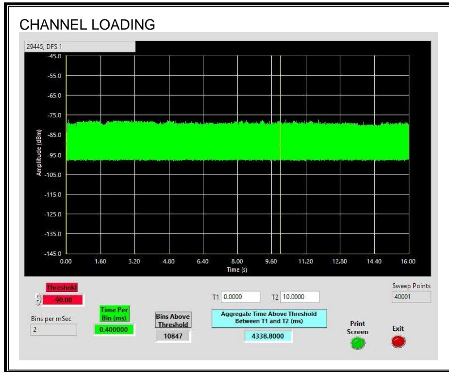
The level of traffic loading on the channel by the EUT is 43.38%
