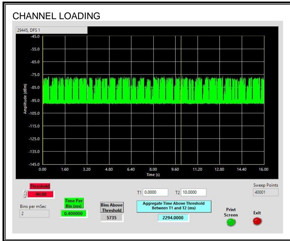
The level of traffic loading on the channel by the EUT is 22.94%
