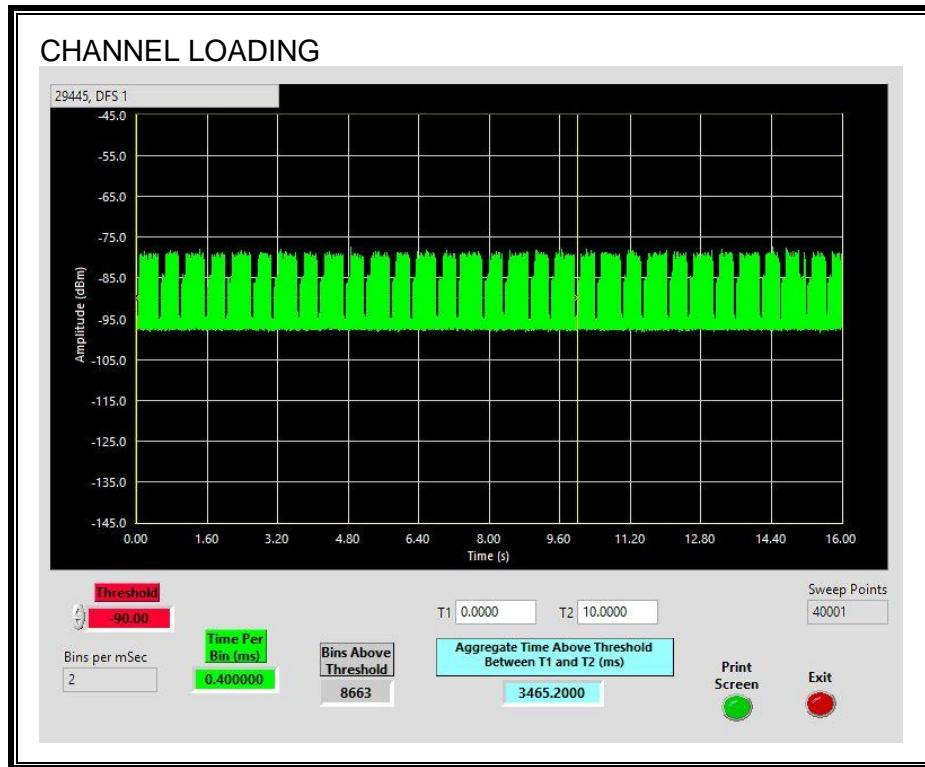
The level of traffic loading on the channel by the EUT is 34.65%
