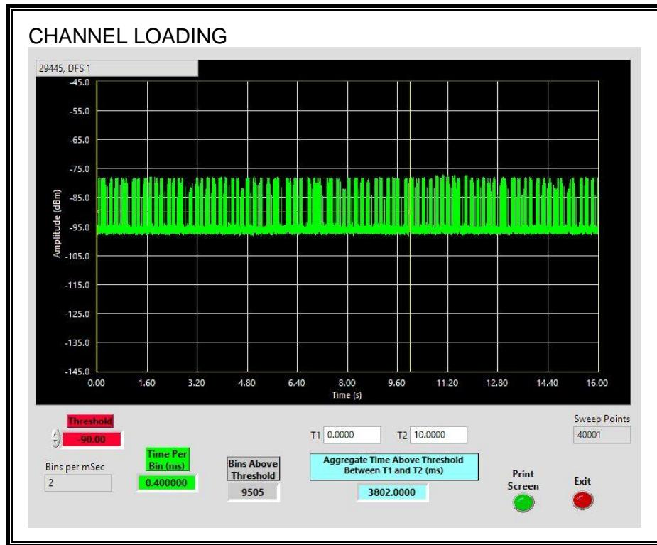
The level of traffic loading on the channel by the EUT is 38.02%
