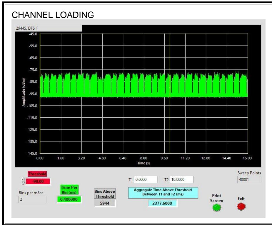
The level of traffic loading on the channel by the EUT is 23.77%
