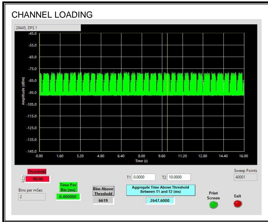
The level of traffic loading on the channel by the EUT is 26.47%
