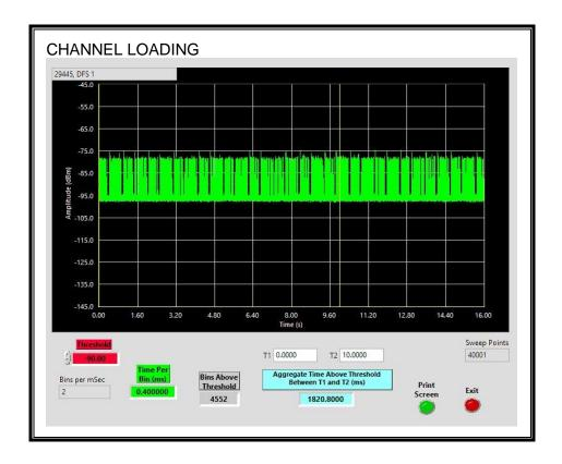
The level of traffic loading on the channel by the EUT is 18.2%
