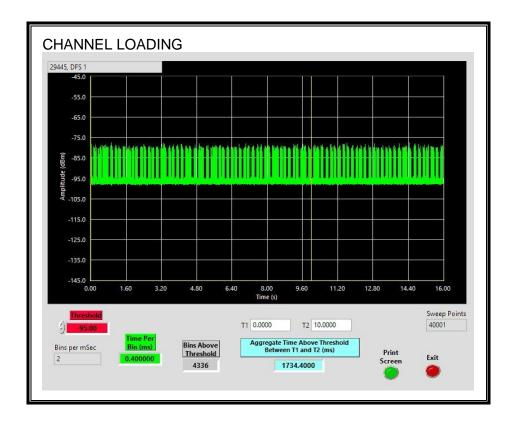
The level of traffic loading on the channel by the EUT is 17.34%
