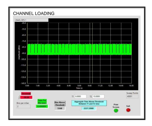
The level of traffic loading on the channel by the Peer Slave is 22.27%
