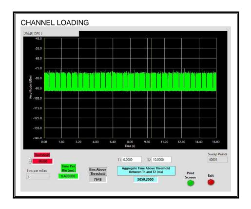
The level of traffic loading on the channel by the EUT is 30.59%
