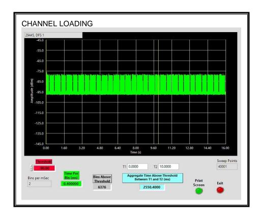
The level of traffic loading on the channel by the Peer Slave is 25.5%
