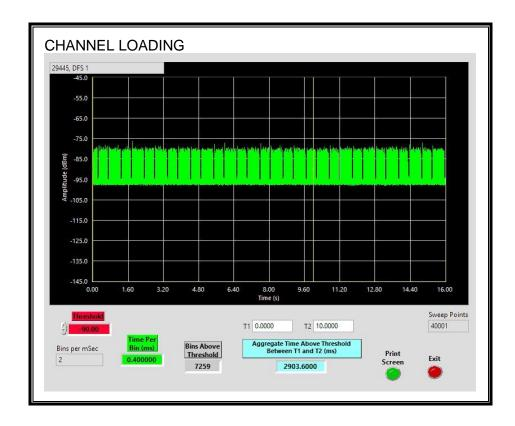
The level of traffic loading on the channel by the EUT is 29.03%
