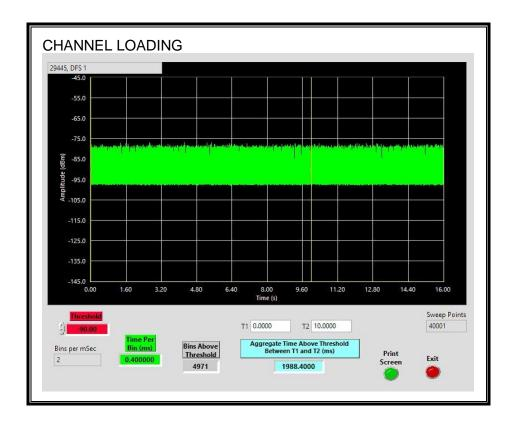
The level of traffic loading on the channel by the EUT is 19.88%
