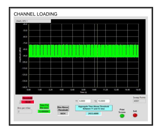
The level of traffic loading on the channel by the Peer Slave is 26.53%
