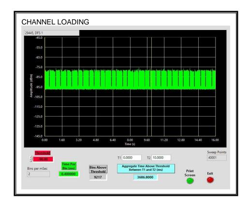
The level of traffic loading on the channel by the EUT is 36.86%
