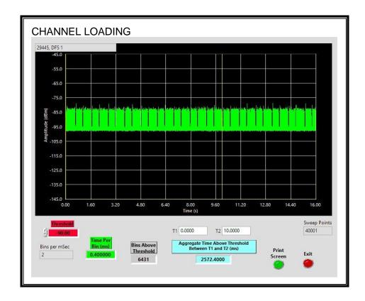
The level of traffic loading on the channel by the EUT is 25.72%
