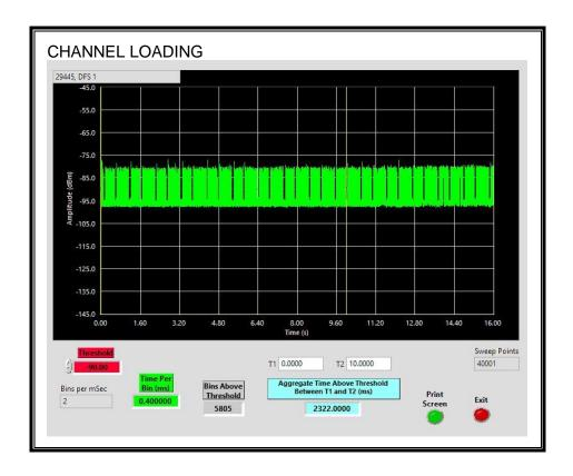
The level of traffic loading on the channel by the EUT is 23.22%
