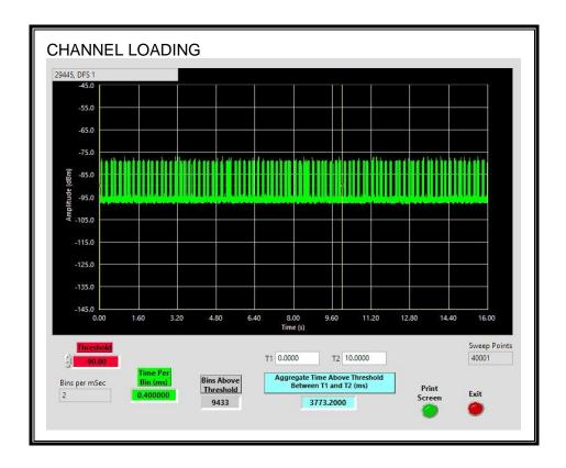
The level of traffic loading on the channel by the EUT is 37.73%
