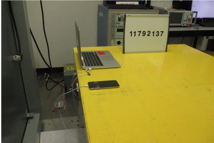
LINE CONDUCTED BACK PHOTO
