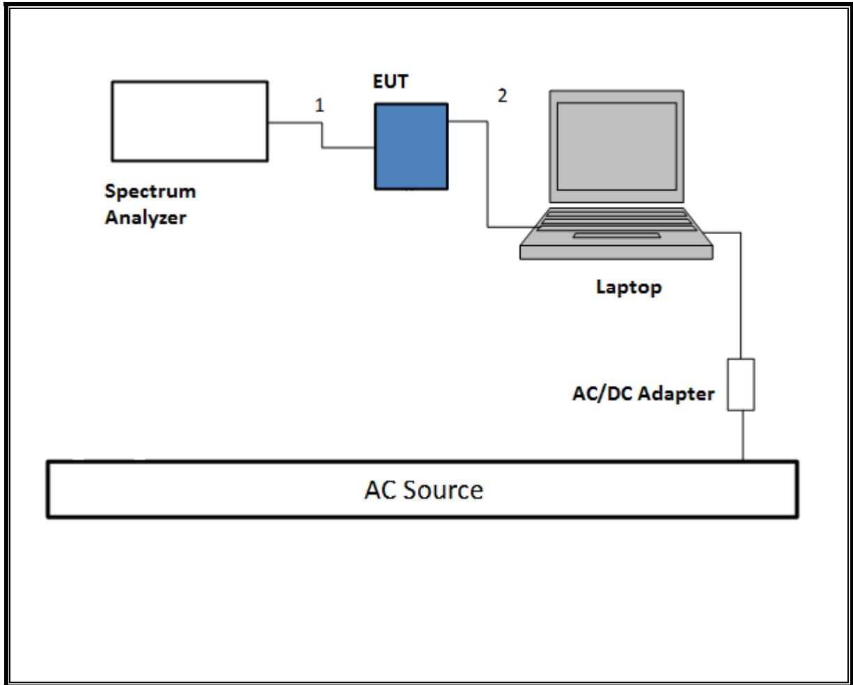
**RADIATED TEST SETUP -ABOVE 1 GHZ**
