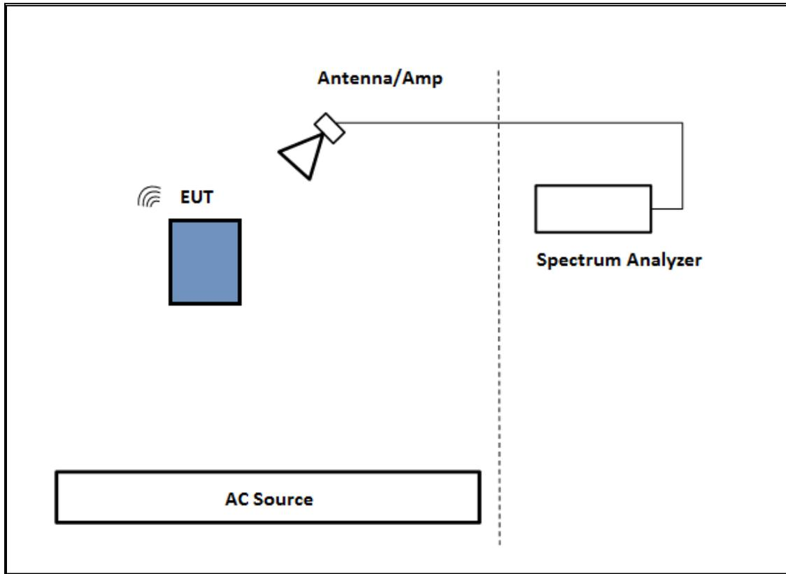
**BELOW 1GHZ & AC LINE CONDUCTED TEST SETUP**
