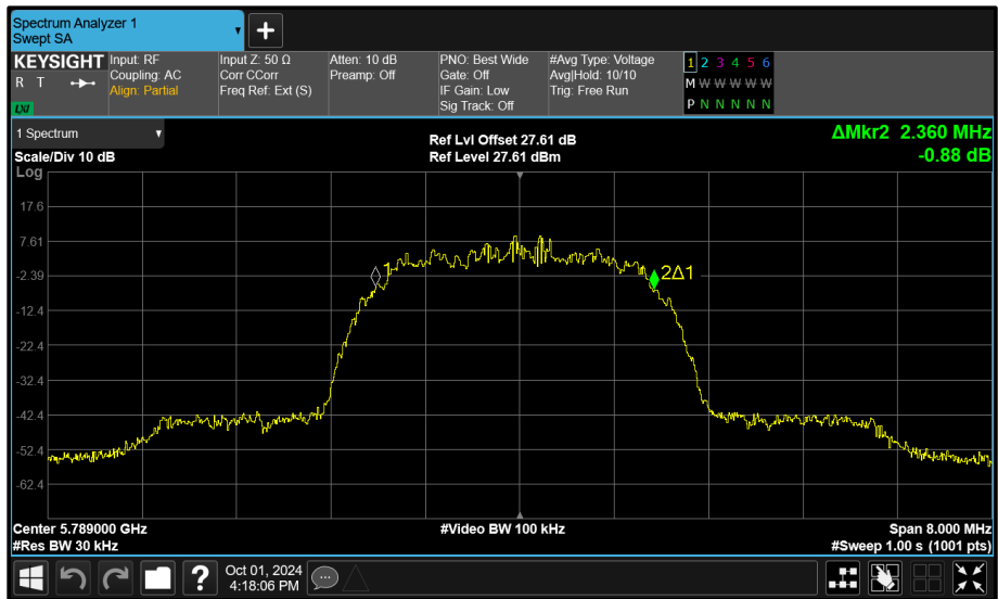
Figure 148 - Core 1 (B) 5789 MHz (CH64) 99% Bandwidth
