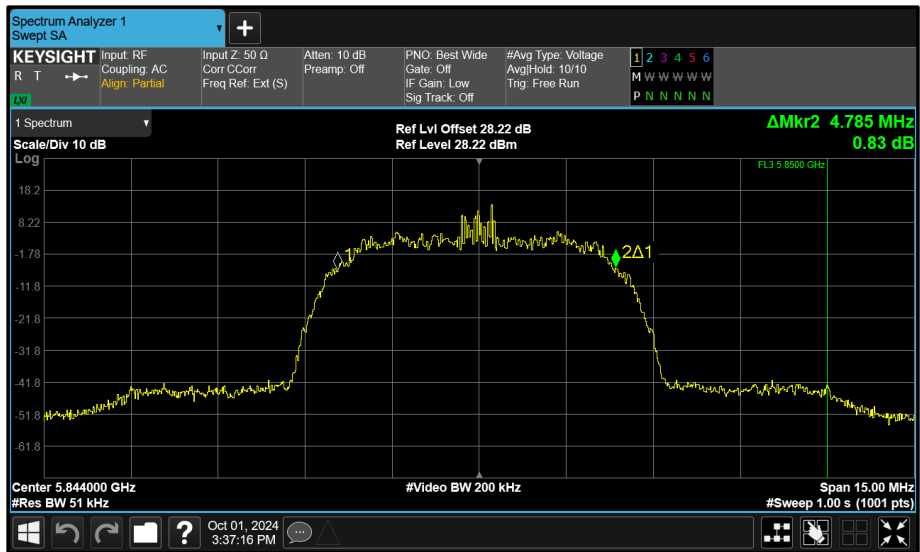
Figure 74 - Core 0 (A) 5844 MHz (CH119) 99% Bandwidth
