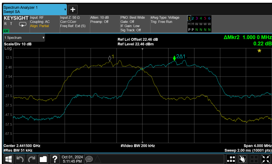
Figure 56 - 8-DPSK - 2441 MHz (CH39) & 2442 MHz (CH40)
