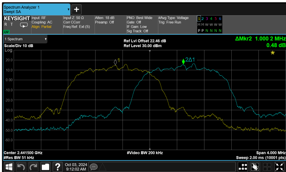
Figure 51 - 8-DPSK - 2441 MHz (CH39) & 2442 MHz (CH40)
