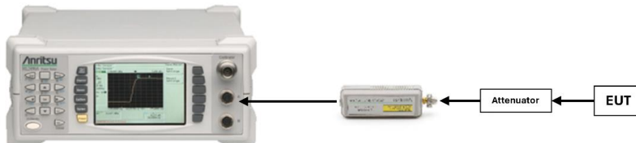
Figure 7-2. Test Instrument & Measurement Setup for Power Meter Measurements
