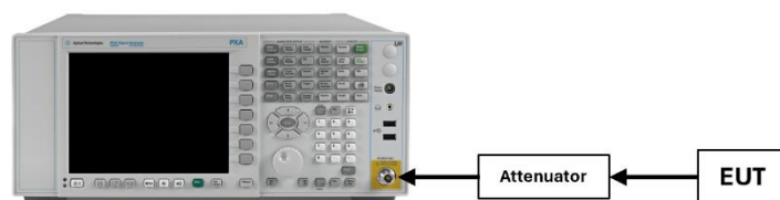
Figure 7-5. Test Instrument & Measurement Setup
