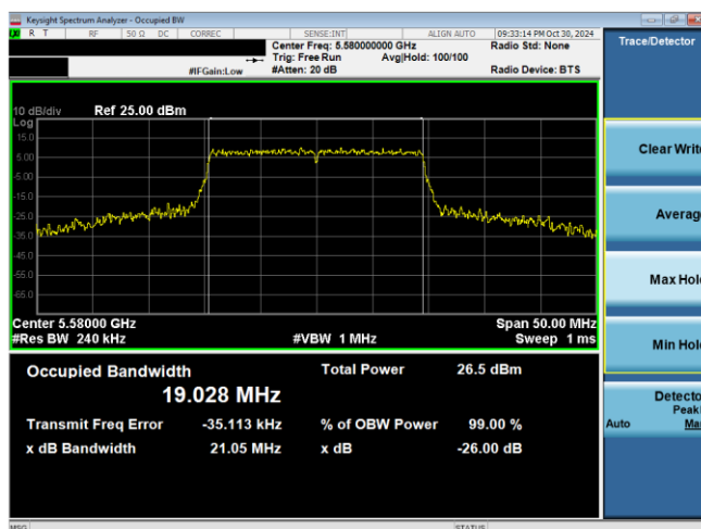
Plot 7-2. 26dB BW & 99% OBW Antenna 3c (20MHz BW 11ax– RU242 – Ch.116)
