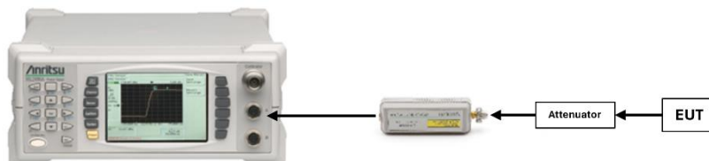
Figure 7-3. Test Instrument & Measurement Setup
