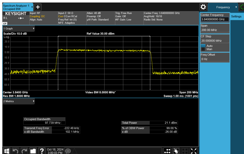
Plot 7-110. Occupied Bandwidth Plot (NR Band n77 C-Band - 100MHz CP-OFDM 256-QAM - Full RB)
