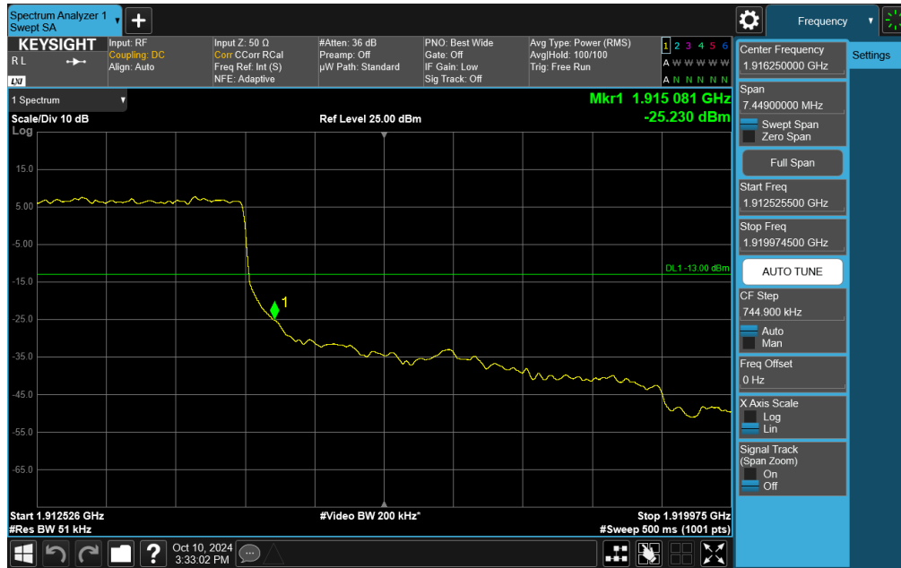
Plot 7-143. Upper Band Edge Plot (NR Band n25 – 5MHz DFT-s-OFDM \pi/2 BPSK – Full RB Configuration)
