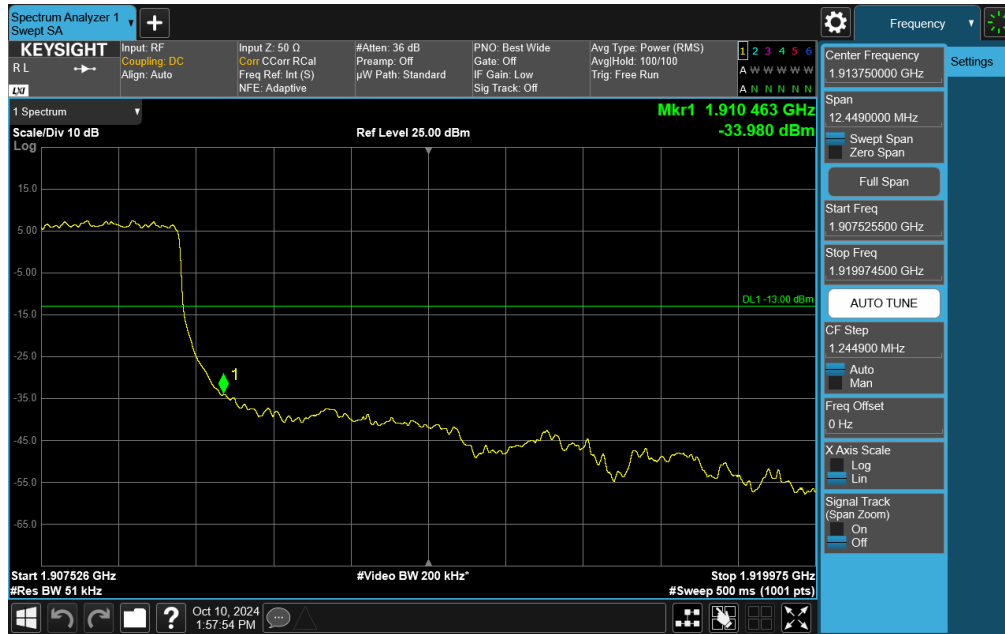
Plot 7-175. Upper Band Edge Plot (NR Band n2 – 5MHz DFT-s-OFDM \pi/2 BPSK – Full RB Configuration)
