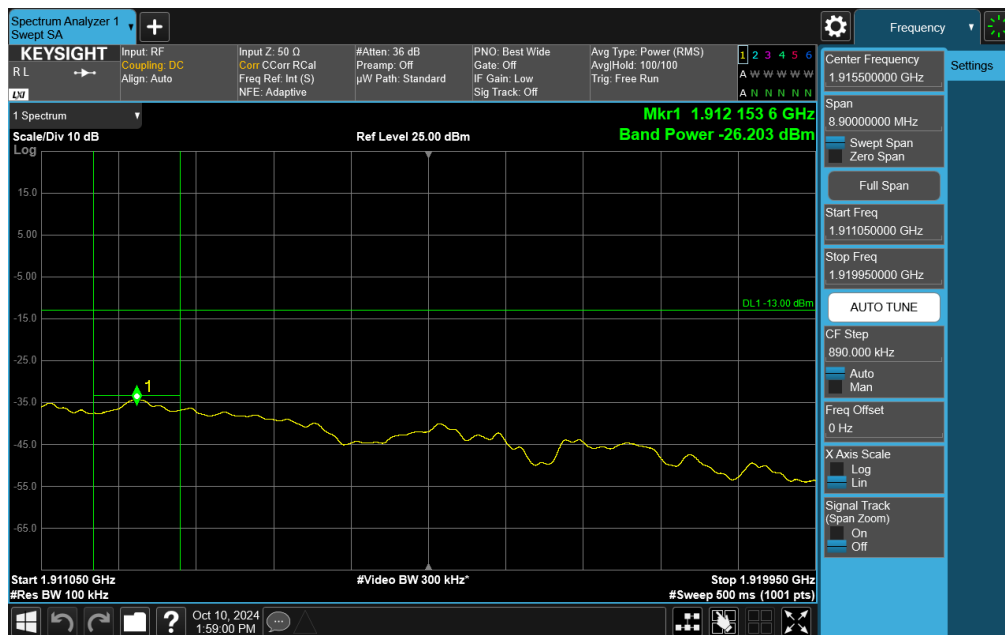
Plot 7-176. Extended Upper Band Edge Plot (NR Band n2 – 5MHz DFT-s-OFDM \pi/2 BPSK – Full RB Configuration)
