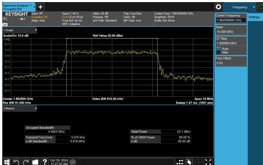
Plot 7-26. Occupied Bandwidth Plot (NR Band n25/n2 - 5MHz CP-OFDM QPSK - Full RB)
