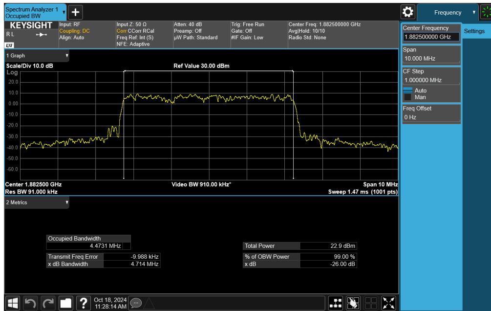
Plot 7-27. Occupied Bandwidth Plot (NR Band n25/n2 - 5MHz CP-OFDM 16QAM - Full RB)
