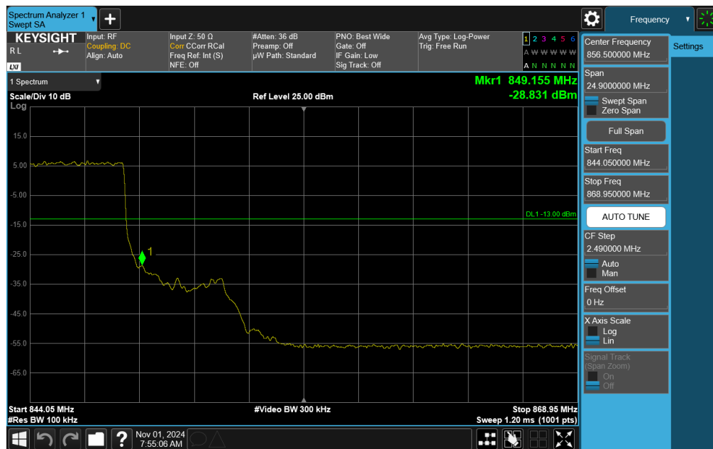
Plot 7-107. Upper BE Plot (NR Band n5 DFT-s-OFDM \pi/2 BPSK – 10.0MHz - Full RB)
