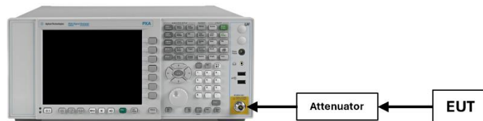
Figure 7-5. Test Instrument & Measurement Setup
