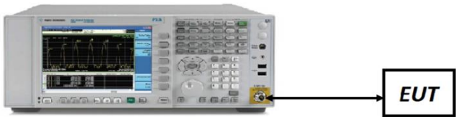
Figure 7-1. Test Instrument & Measurement Setup
