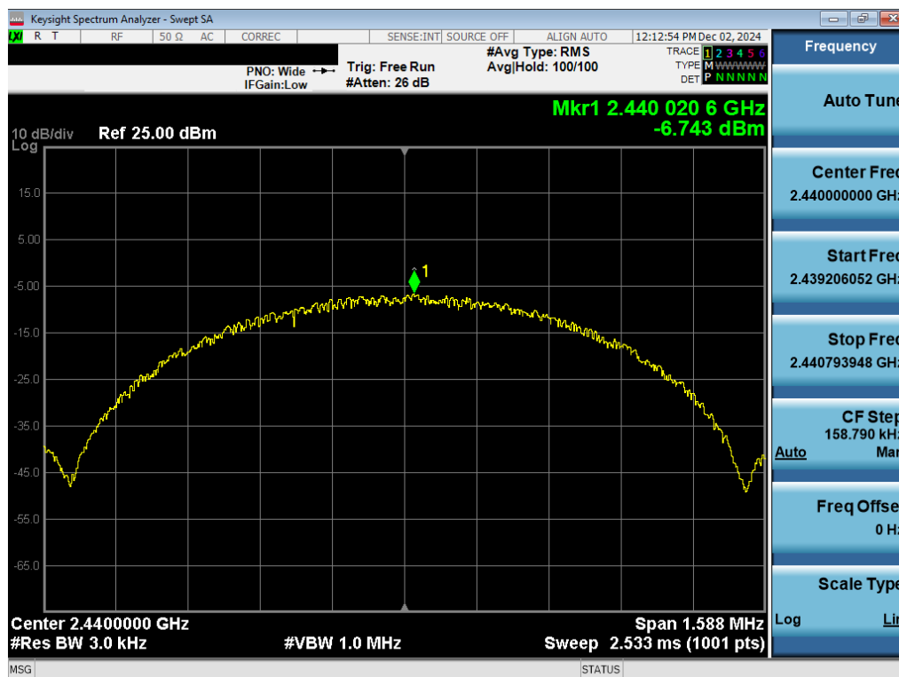
Plot 7-46. Power Spectral Density Plot Antenna WF2b (Bluetooth (LE), 1Mbps, iPA – Ch. 19)
