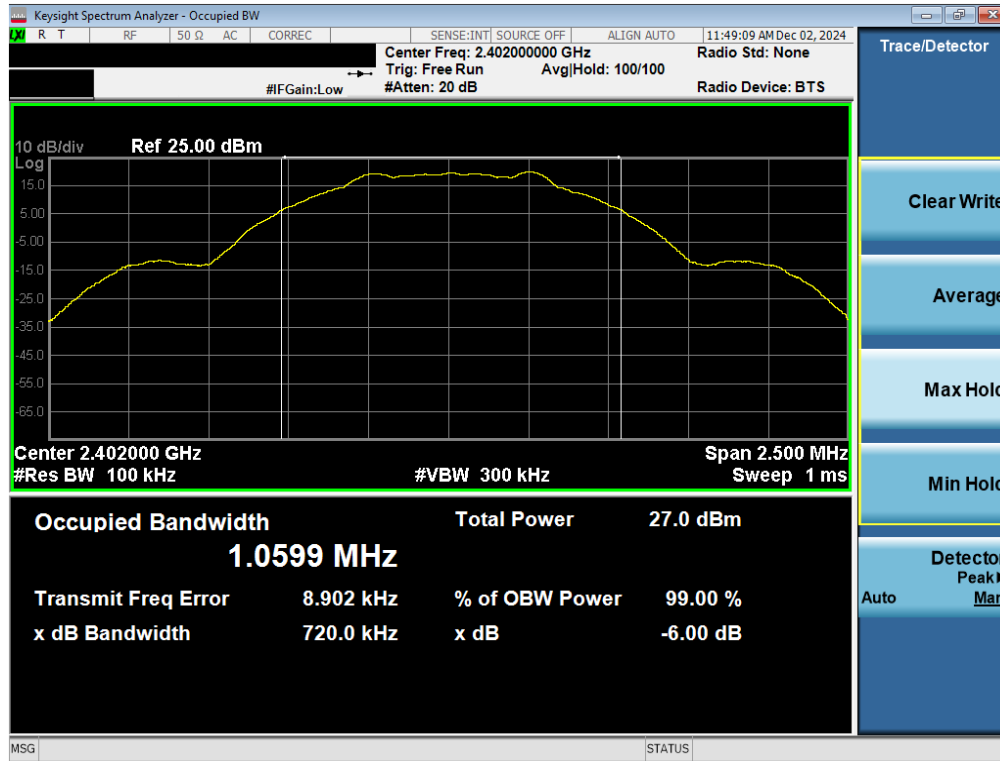
Plot 7-7. 6dB BW & 99% OBW Plot Antenna WF2b (Bluetooth (LE), 1Mbps, ePA – Ch. 0)
