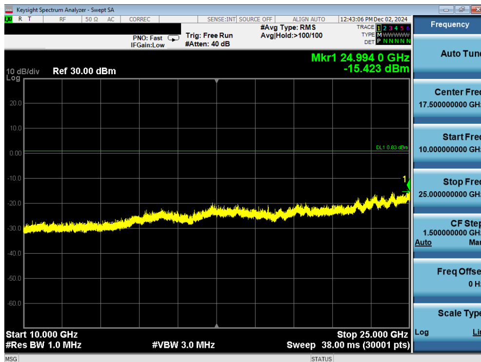
Plot 7-76. Conducted Spurious Plot Antenna WF2b (Bluetooth (LE), 1Mbps, ePA – Ch. 0)
