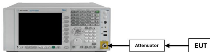
Figure 7-3. Test Instrument & Measurement Setup
