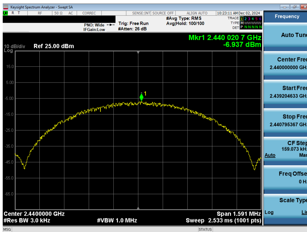
Plot 7-45. Power Spectral Density Plot Antenna WF7b (Bluetooth (LE), 1Mbps, iPA – Ch. 19)
