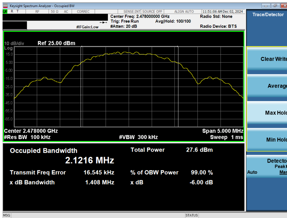
Plot 7-12. 6dB BW & 99% OBW Plot Antenna WF2b (Bluetooth (LE), 2Mbps, ePA – Ch. 38)
