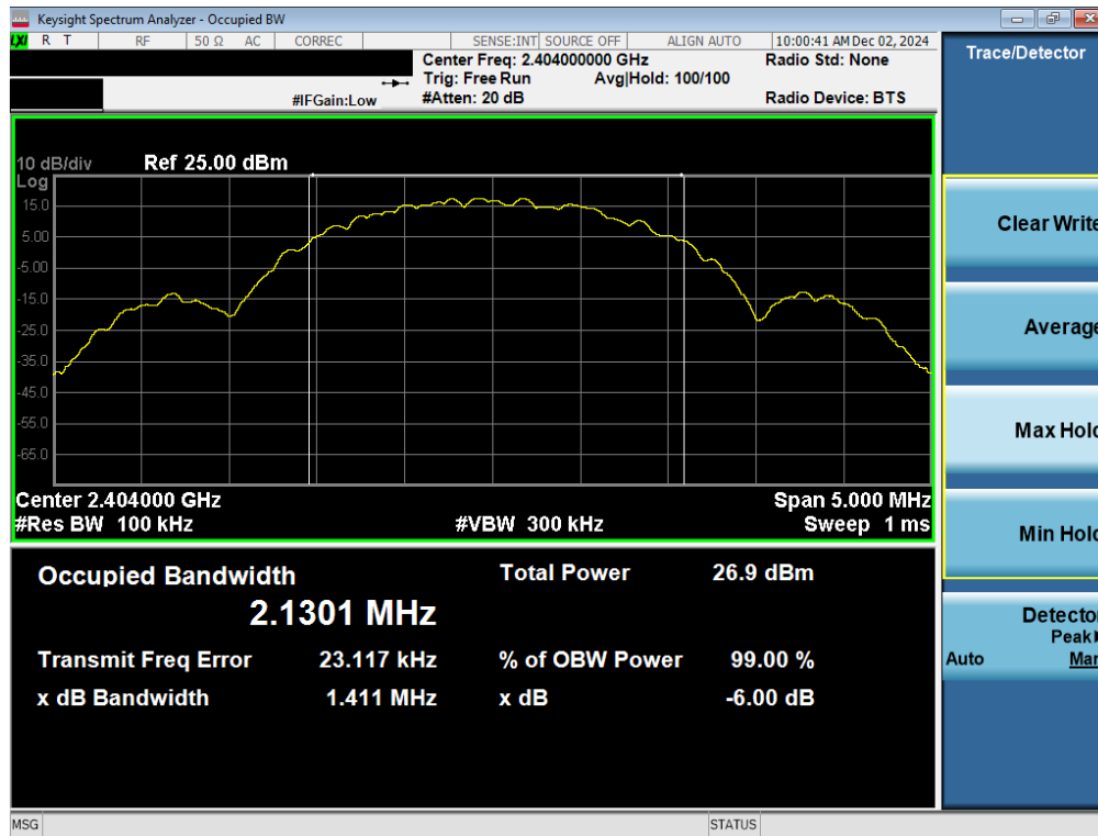
Plot 7-4. 6dB BW & 99% OBW Plot Antenna WF7b (Bluetooth (LE), 2Mbps, ePA – Ch. 1)
