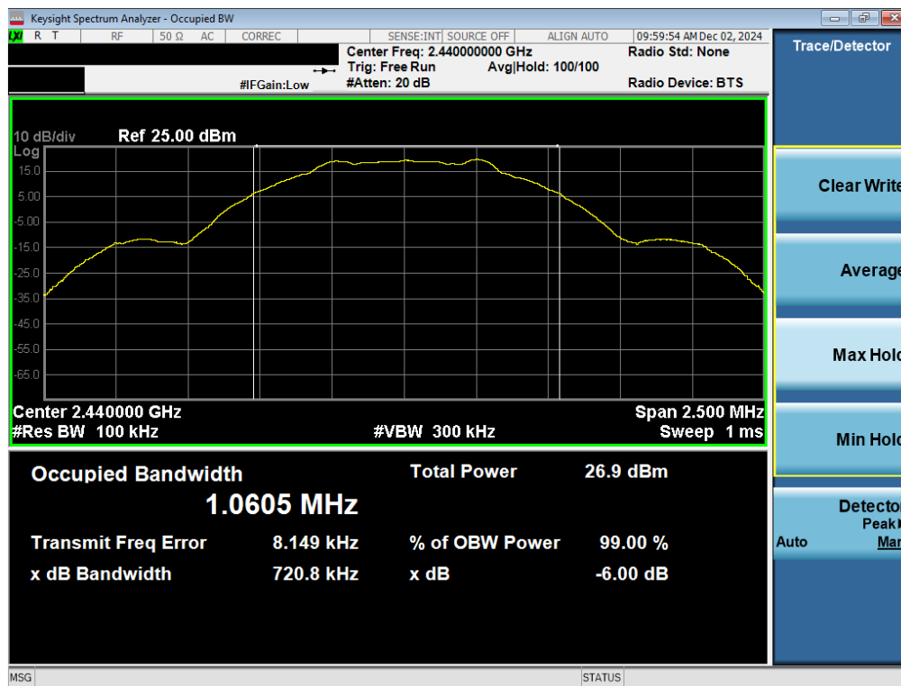
Plot 7-2. 6dB BW & 99% OBW Plot Antenna WF7b (Bluetooth (LE), 1Mbps, ePA – Ch. 19)
