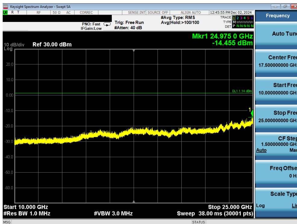
Plot 7-80. Conducted Spurious Plot Antenna WF2b (Bluetooth (LE), 1Mbps, ePA – Ch. 39)
