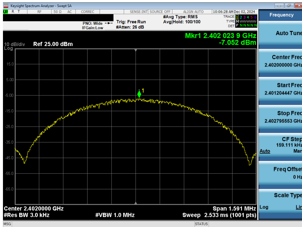
Plot 7-16. Power Spectral Density Plot Antenna WF7b (Bluetooth (LE), 1Mbps, iPA – Ch. 0)
