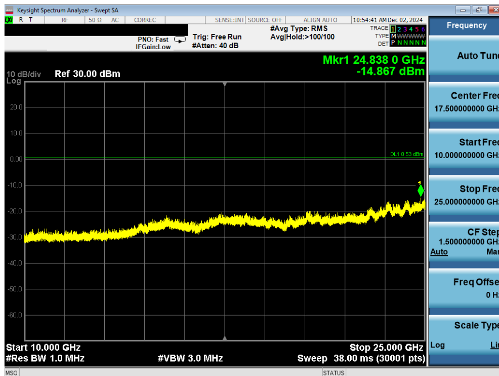
Plot 7-72. Conducted Spurious Plot Antenna WF7b (Bluetooth (LE), 1Mbps, ePA – Ch. 19)
