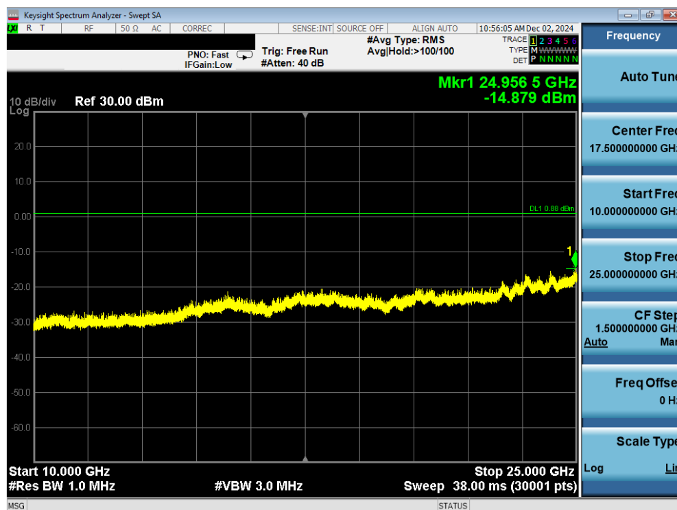
Plot 7-74. Conducted Spurious Plot Antenna WF7b (Bluetooth (LE), 1Mbps, ePA – Ch. 39)
