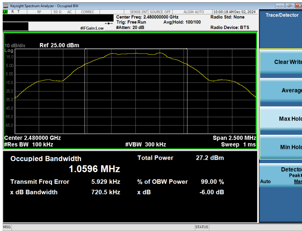
Plot 7-3. 6dB BW & 99% OBW Plot Antenna WF7b (Bluetooth (LE), 1Mbps, ePA – Ch. 39)
