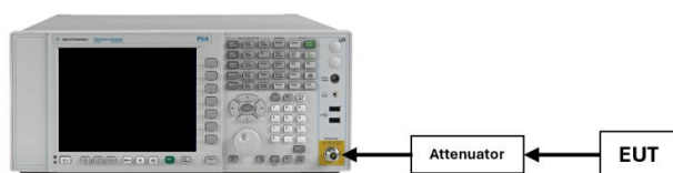
Figure 7-4. Test Instrument & Measurement Setup
