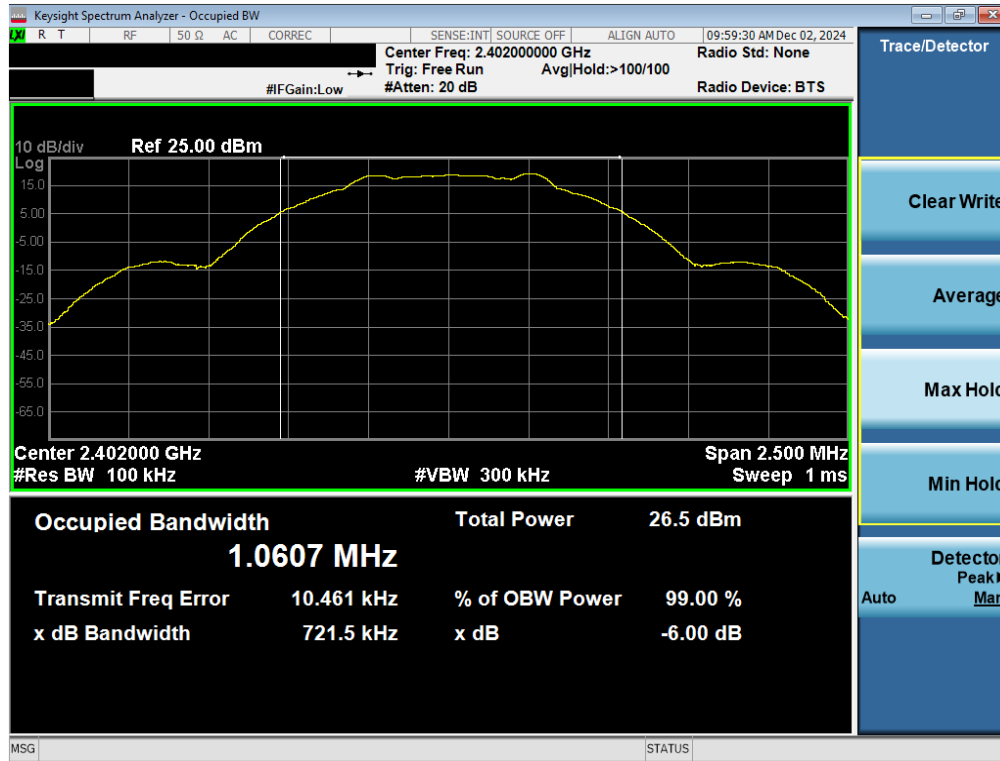
Plot 7-1. 6dB BW & 99% OBW Plot Antenna WF7b (Bluetooth (LE), 1Mbps, ePA – Ch. 0)
