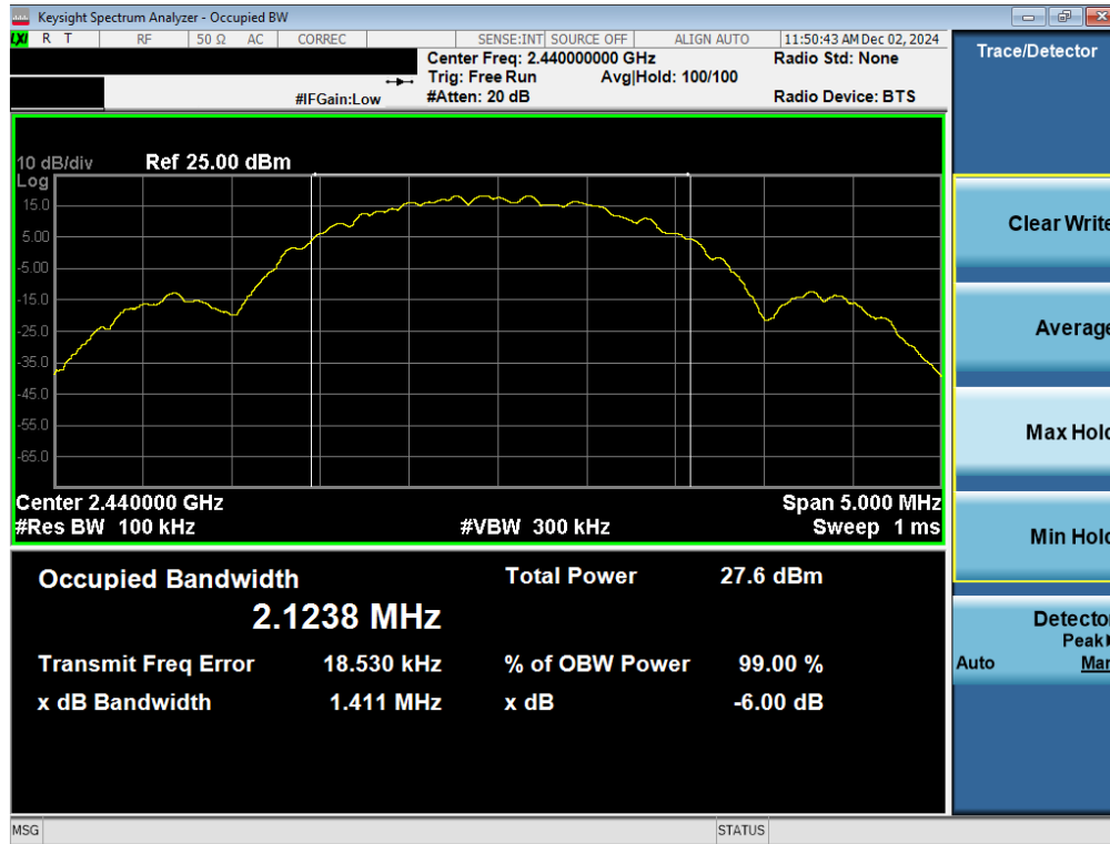
Plot 7-11. 6dB BW & 99% OBW Plot Antenna WF2b (Bluetooth (LE), 2Mbps, ePA – Ch. 19)
